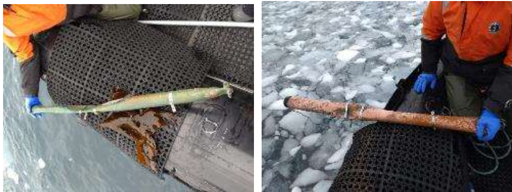
Figure 2- Before and after grounding pipe cleaning
